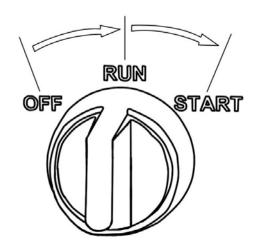
The battery is working for the carburetor valve at "RUN" channel. So please make sure the switch is at the "OFF" channel when the unit is turn off.
