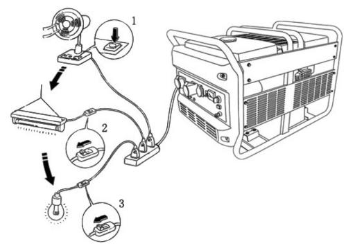
In general, the capacitive load or inductive load will need great starting current, when it turns on, specially the motor actuating device. The following table indicates the parameter of the appliances for your reference:
